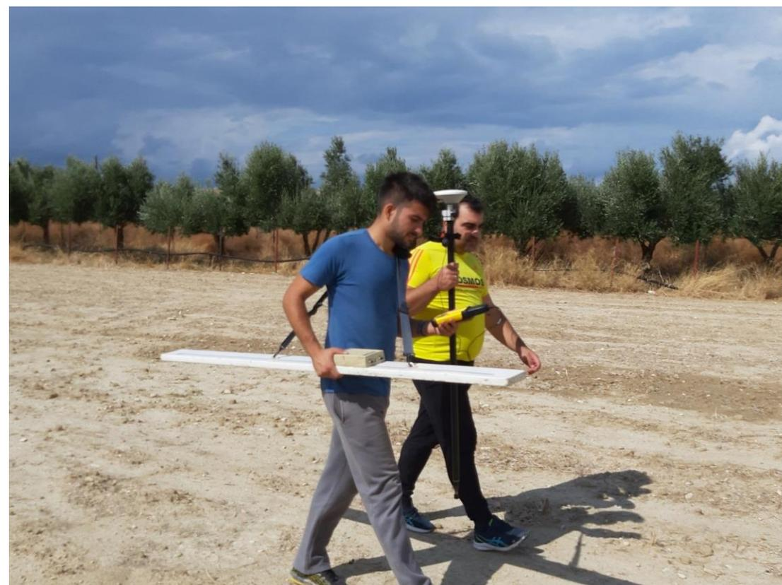
Mapping conductivity in an agricultural field near to a stream using GEM-2 sensor and GPS
