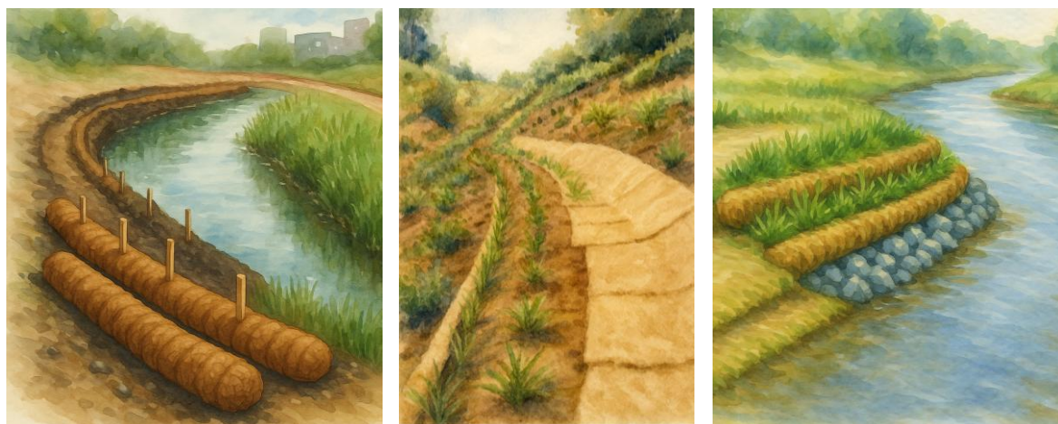
Figure 32. Illustration examples of fibre rolls, mats, and pallets made from fibre (e.g., coconut) used for erosion control, soil stabilization, and vegetation establishment along slopes and streambanks.
