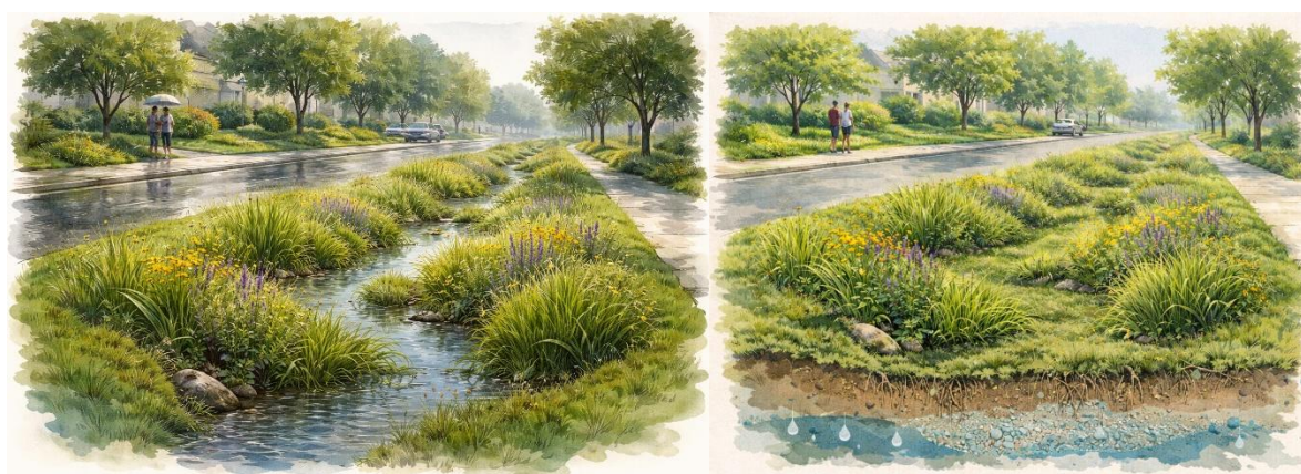
Figure 40 Vegetated swales under contrasting conditions. Vegetated swales illustrated during a rainfall event (left) and under non-rain conditions (right). During rainfall, runoff from adjacent impervious surfaces is conveyed at low velocity, promoting infiltration and pollutant retention. Under non-rain conditions, the swale functions as a vegetated green infrastructure element, providing ecological and aesthetic benefits while remaining integrated into the urban landscape.
