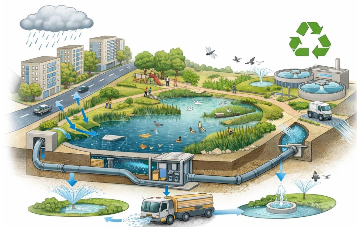
Figure 55. Schematic representation of how a floodable park such as La Marjal operates within an urban environment.
