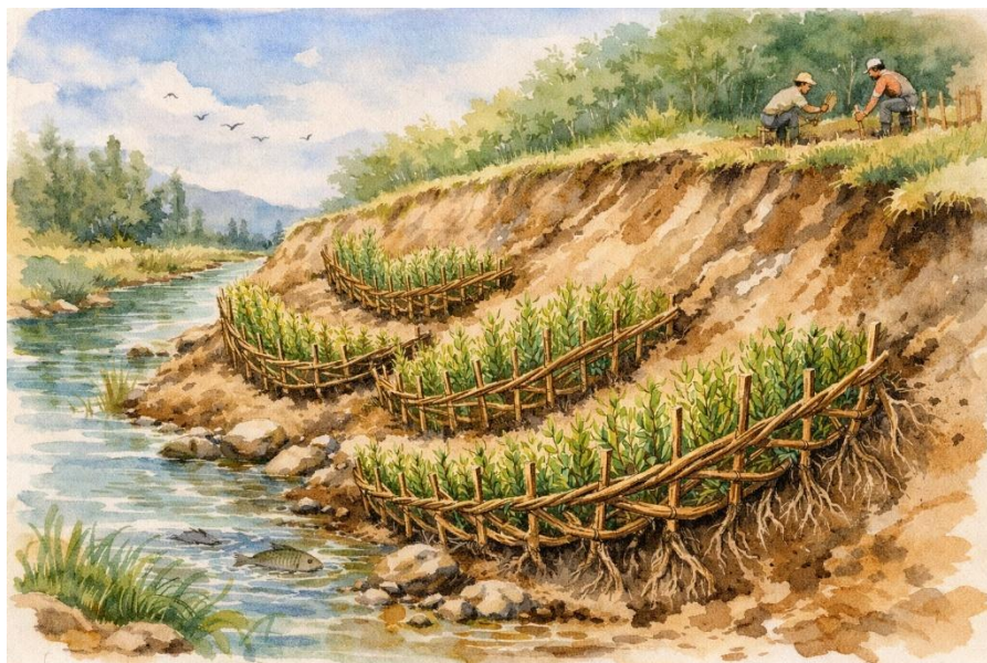
Figure 29. Live smile, many can be done side by side, stabilizing stream banks by combining structural elements with living vegetation, reducing erosion, enhancing habitat complexity, and promoting long-term natural bank resilience. For real examples see Polster (2002) .
