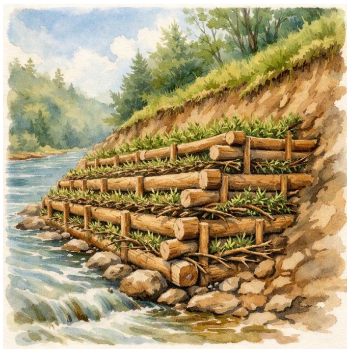
Figure 31. Illustration of a live crib wall combining timber framework and live branch cuttings to provide structural and vegetative stabilization of a steep streambank.
