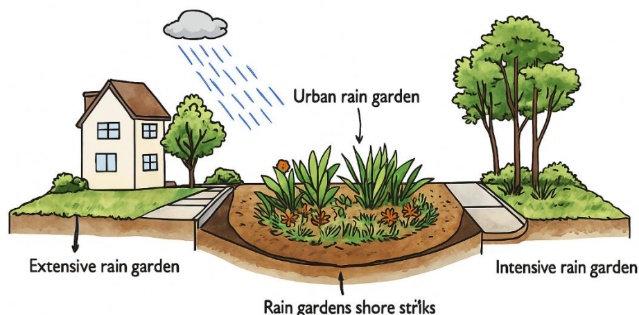
Figure 36. Rain gardens that are designed to capture and absorb stormwater runoff.
