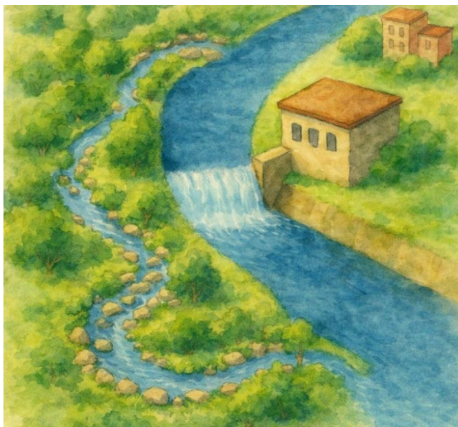
Figure 8. Nature-like bypass channel, mimicking a natural stream morphology, providing ecological continuity, and enhancing aquatic habitat diversity in a restored river reach.
