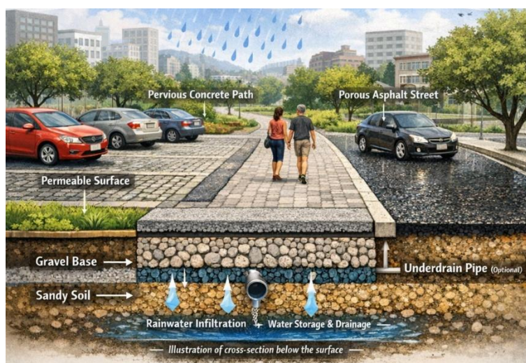
Figure 38. Illustration of permeable pavement systems and their functionality.
