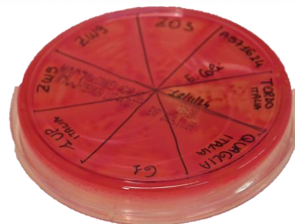
Agar plate showing the colonies of fecal coliforms and enabling their quantification.
