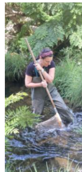
Sampling by kick and sweep upstream sediment by foot with a hand-net
